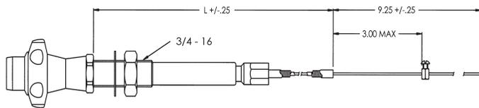
This control allows for precise setting of the engine RPM when the PTO is engaged or as a manual control of the idle position during engine warm up (Friction Lock optional).
