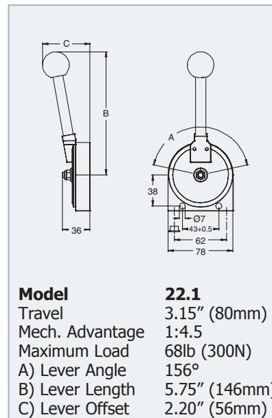
Travel can be limited symmetrically or asymmetrically, on both 22.1 and 22.3 levers, 10/20mm using coiled spring pins (sold separately). Coiled Pin P/N 175-420-034
