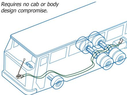
*The cables can easily be routed to avoid displacing valuable luggage space.*
