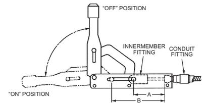
1. Dimension A is with the lever in full "OFF" position. Use dimension A in calculating cable length.
