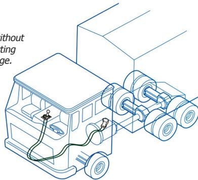
*Cab sealed around shift linkage.*
