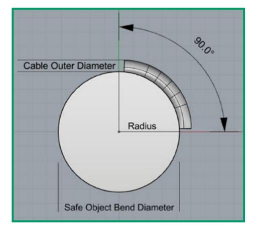
When choosing the right cable for your application, the smaller the bend radius, the more flexible a cable needs to be. If the bend radius is larger, the cable can be less flexible.
